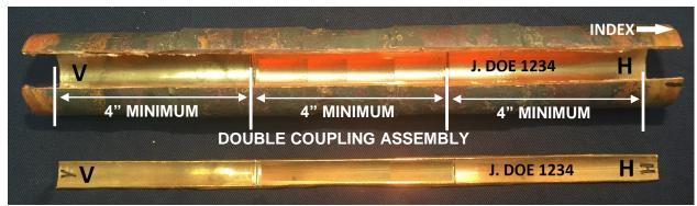
Illustrations are from BTS15 Medical Gas Initial Braze Test – Coupons may be cut in halves or straps. Entire coupon must be submitted. All components must be identified.
